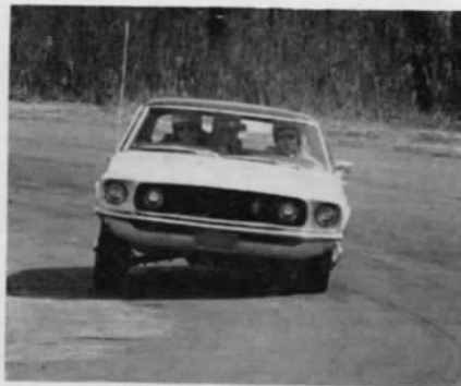
The Mustang handled much better in high-speed turns than the Cougar , understeering less and responding better
