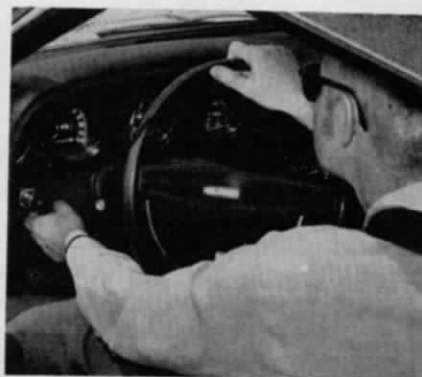
In both Mustang and Cougar , many vital operating controls are beyond the reach of drivers wearing shoulder belts
