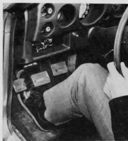
Above: Once you let your left foot get down below the AMX's parking-brake pedal and clutch pedal, you may have trouble getting it out when you need it
