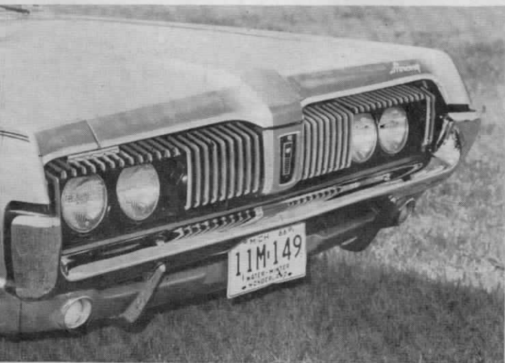
Dual headlamps remain stationary while doors hinge upward and inward, adjustment and aiming remaining undisturbed.
