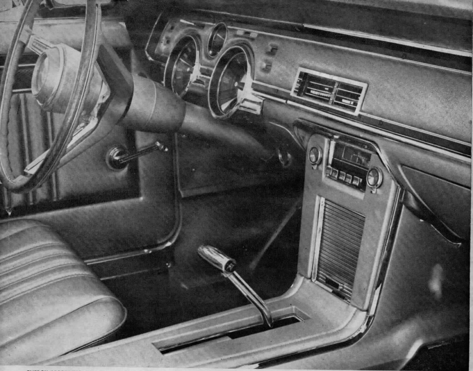
ENERGY-ABSORBING PADDED STEERING WHEEL HUB IS CALLED A "DAGMAR." T-BIRD-LIKE CENTRAL CONSOLE IS OPTIONAL AT EXTRA COST.
